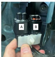
20. Plug in the provided adapters and run the harnesses to the end of the toggle harness from step 12. Disconnect the switch from the standard harness leaving only the 3-pin white connector. Connect the two harnesses using the appropriate connector from the list below. Tie away any slack using the zip ties provided.
